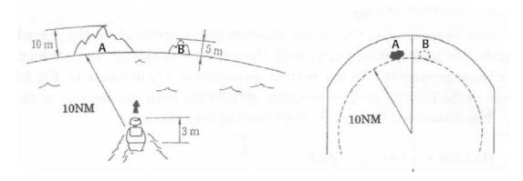
In this example, the scanner is installed on the vessel at a height of 10 ft (3 m) above sea level (h1). Island A is 33 ft (10 m) high (h2) and for comparison, Island B is 16.4 ft (5 m) high (h2). Both islands are at a distance (D) of 10 nautical miles from the vessel.
